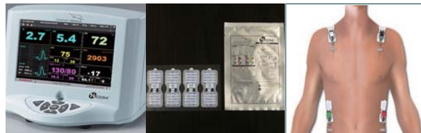
Figure 1. Monitor and electrodes for the bioreactance noninvasive cardiac output monitoring method
