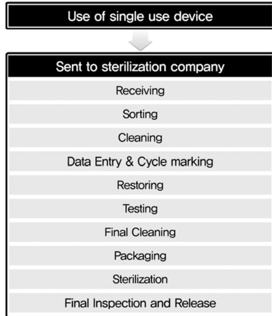
Figure 3. US Sterilization Process
